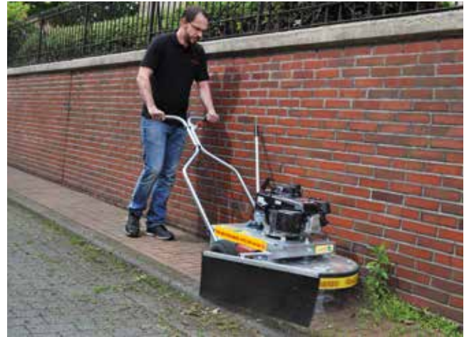
The windrow maker / splash back can be mounted toolless.
