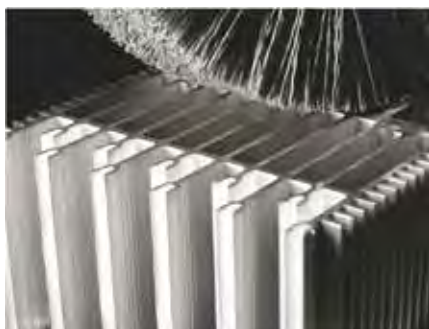
Sbavare oggetti estrusi in alluminio / Deburring of extruded aluminium profiles
