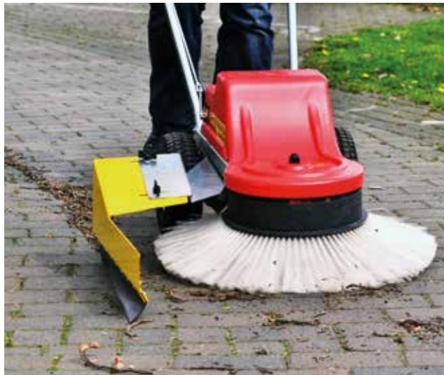
With the windrow maker, large-volume and long-fiber dirt can be dropped into a windrow.
